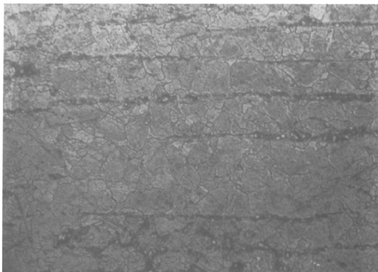
Fig. 6. Strip section of Pb-1.8wt.%Sb-0.15wt.%As-0.2wt.%Sn alloy ( \times 160 ).
